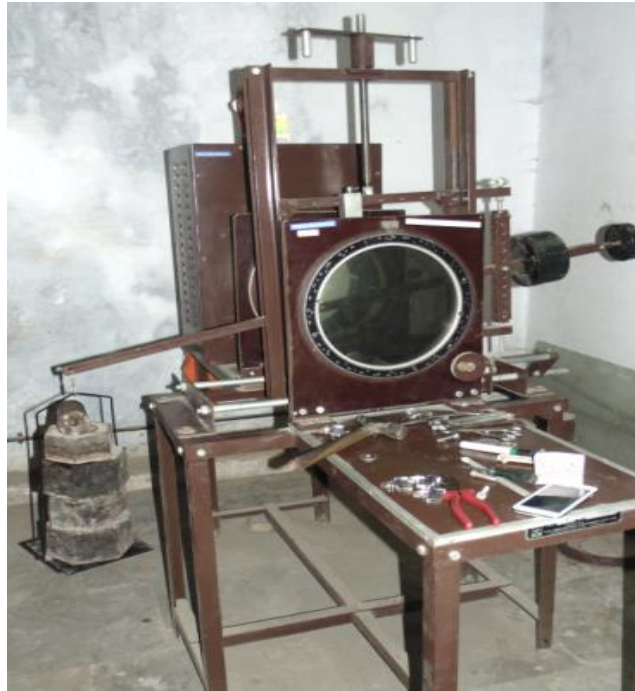
Fig. 6.1 Diffused light Polariscope
