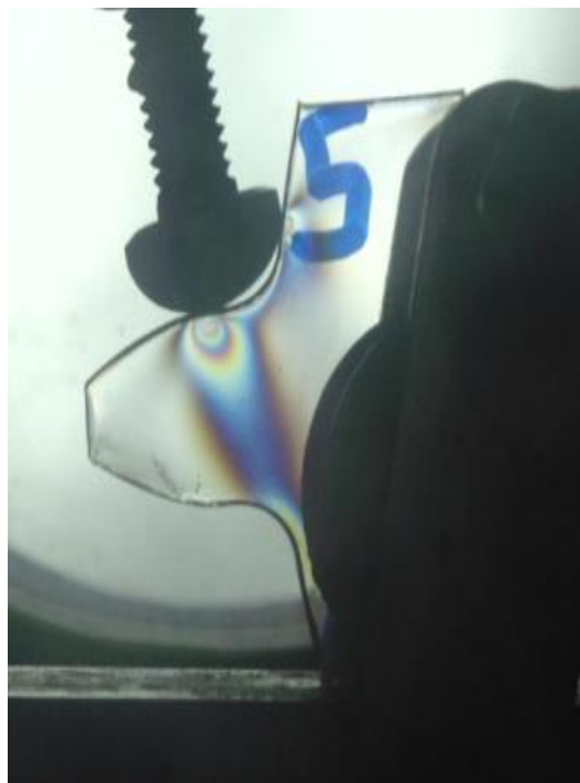
Symmetric gear Pressure angle 20^{\circ} - 20^{\circ} Load applied = 35 kg Test Specimen 5
